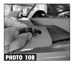
**10.** Place the grille back into position and snap in the lower clips (See Photo 10A), then place the six upper clips back into place. (See Photo 10B)
