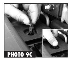
**9C** Insert the two clips back into position and push them down into place. (See Photo 9C)
