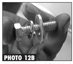
**12B & 12C.** Using the supplied bolts, lock washers, and flat washers (See Photo 12B), insert them through the bracket and into the bottom side of the tube, but only make them finger tight. (See Photo 12C)
