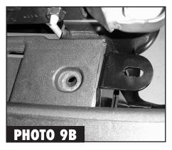
**9A & 9B.** Reinsert the bumper spacer plate back into position and align the clip holes. (See Photos 9A & 9B)
