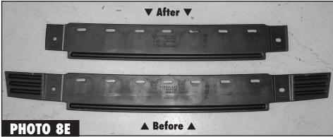
8. Measure and mark on both sides of the bumper spacer plate 3-1/4" from the inside kick out. (See Photos 8A & 8B) Using a cutting tool make both cuts at the marked line. (See Photos 8C & 8D) This is a before and after of your bumper spacer plate. (See Photo 8E)
