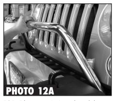
**12A.** Take your new Pre-Runner bar and align it up with the holes in the bracket. (See Photo 12A)
