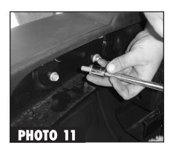
**11.** Replace the tow bolts and two nuts from each side of the bumper and tighten. (See Photo 11)
