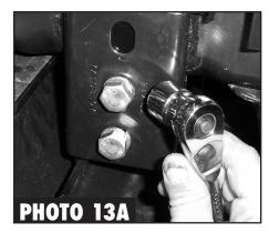
**13A.** Now tighten up the two bracket bolts on each side. (See Photo 13A)
