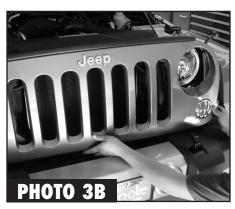
**3B.** Repeat this on the other side then pull outwards towards the center removing the last 4 clips. (See Photo 3A)
