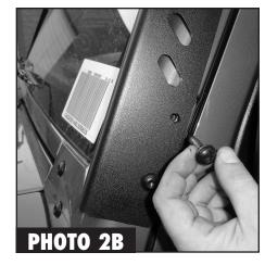
**2.** Align the mounting brackets with the flat edge facing forward and the form facing the middle of the vehicle (See Photo 2A). Replace the factory bolts and finger tighten them (See Photo 2B).
