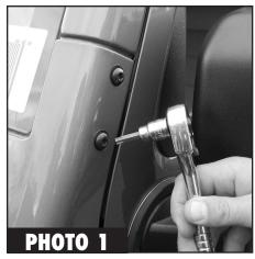
**1.** Begin by removing the top two bolts along the outer windshield mount on both sides by using a T-40 torx bit (See Photo 1).
