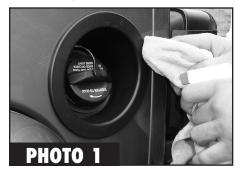
**1. Extremely Important: Clean the area where the Fuel Door is to be installed.** If the area where the Fuel Door is to be installed is not clean, dry, and free of any vinyl dressing, the Fuel Door will not stick in place. Begin by cleaning the area thoroughly with a good non-residue cleaner such as Windex, or just clean thoroughly with soap and water and dry completely.
