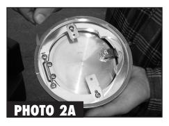
**2.** Open the fuel door slightly and peel the 3M tape backing (See Photo 2A). Align over the fuel bucket (See Photo 2B). Make sure that the fuel door is level and centered correctly, then push firmly against the body of the vehicle (See Photo 2C).
