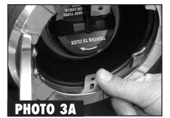
3. Now press the bottom and top tabs firmly against the fuel bucket (See Photos 3A, 3B & 3C).
