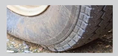
Never reinflate a tire that has operated in a run-flat condition or at 80% or less of recommended operating pressure.
