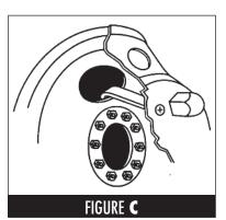
Line up the mounting hooks on the back of the wheel simulator with the hand holes of the wheel. (See Fig. B).
