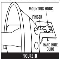
"ODD" number of hand holes in the wheel. The number of hand holes in the wheel determines the correct Hook Mount System you will need to properly install your Rear wheel simulators (See Figure A).
