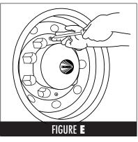
**Very Important:** After initial installation, the mounting system will seat itself into the wheel. After the first 100 miles check that the simulators are tight and secure to the wheels. If necessary retighten the mounting screws. We recommend that the wheel simulators are checked and inspected periodically to make sure that they are tight and secure to the wheels.
