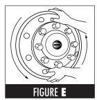
readjust the simulator so that it is centered around the rim, then repeat the tightening procedure in Step 3.
