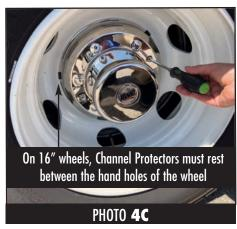
**Note for 16" Installation Only:** To protect the rim on 16" wheels, you'll need to slide on three rubber Channel Protectors evenly spaced on the bottom edge of each Hub Cover. The provided Channel Protectors **must** rest between the hand holes of the wheel rim. (See Photo 4C) Test fit the Hub Cover aligning holes in Cover with holes in the brackets to determine correct position of the Channel Protectors so they will rest between the hand holes.
