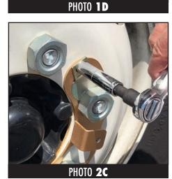
Step 2. Installing Bracket Locking Tabs
