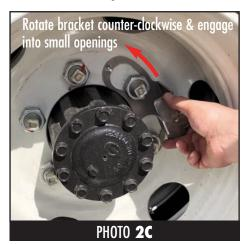
**Step 2. Installing Brackets**—**Note:** Your bracket may differ slightly from photos. Same general instructions still apply. **Note:** Do not remove lug nuts. Larger openings of bracket base will clear lug nuts.
