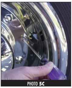
Then use a phillips head screwdriver to securely tighten the bolts. (See Photo 5C)
