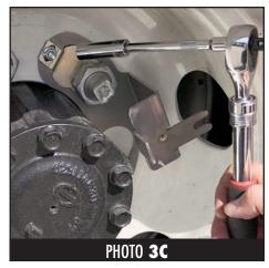
**Step 3.** Installing Bracket Locking Tabs
