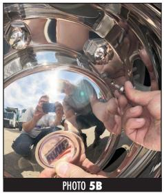
Thread bolts with star washers (provided) through Simulator and into bracket holes. (See Photo 5B)
