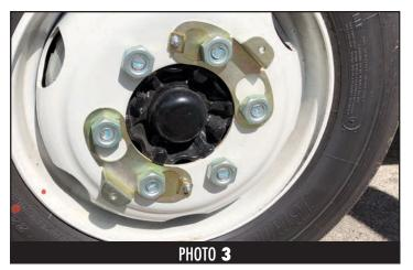
STEP 4. Installing the Simulator onto the Brackets
