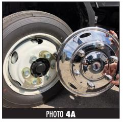
Align holes in Simulator with the holes in the bracket. Make sure the simulator is held up and evenly spaced around the rim edge. (See Photo 4A)
