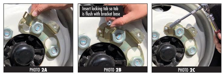
Step 2. Installing Bracket Locking Tabs
