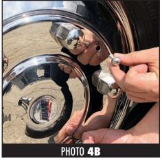
Thread bolts with star washers (provided) through Simulator and into bracket holes. (See Photo 4B)
