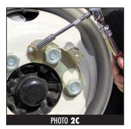
Step 2. Installing Bracket Locking Tabs
