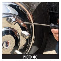
Then use a phillips head screwdriver to securely tighten the bolts. (See Photo 4C)
