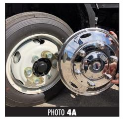
Align holes in Simulator with the holes in the bracket. Make sure the simulator is held up and evenly spaced around the rim edge. (See Photo 4A)
