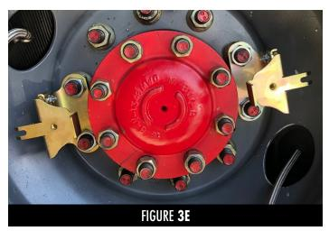
Step 4. Attaching Air Valve Extentions to Air Valve Tabs (Optional)
