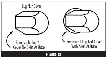
**Important Note:** To remove the covers for inspection, reverse the process by locating the two lug nut covers that do not have skirts at their bases (See Figure D). Remove them, unscrew the two mounting nuts and then remove the wheel cover.
