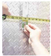
**2. Center** Using the back plate as a template, center/position the back plate in the desired location.
