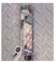
**6. Secure** Place back plate onto bolt studs on the back of the mounting area and secure with washers and nuts.
