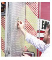
**1. Position** For bracket mounting, identify a flat area on the truck which also has rear access to tighten bolts.
