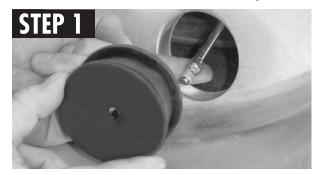
Place the rubber valve stem stabilizer up to the valve extension and align the stabilizer's center hole with the valve extension tip.
