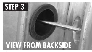
If possible, check between the duals to make sure the flange of the stabilizer has come through the hole in the backside of the wheel and is seated around it.
