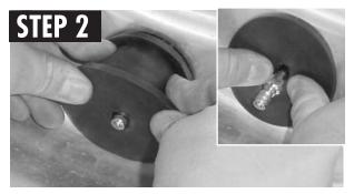
Continue pushing the rubber stabilizer into the wheel hole until the stabilizer's front face is completely seated onto the face of the wheel.
