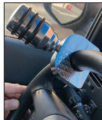
**Step 5.** Place the Top Clamp with Spinner Knob on the steering wheel in the desired location.
