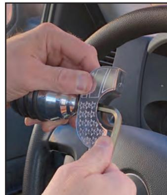
**Step 1.** Using a 3/16" Allen Wrench remove the two bolts from the bottom clamp and separate the two halves.
