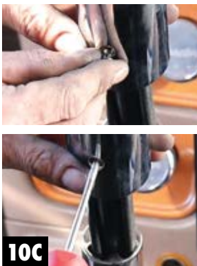
Step 10 Slide Up the Base Cover • Slide up the base shift cover (See Fig. 10A & 10B). Install the 2 Torx T20 screws that were taken out of the old base cover (10C).
