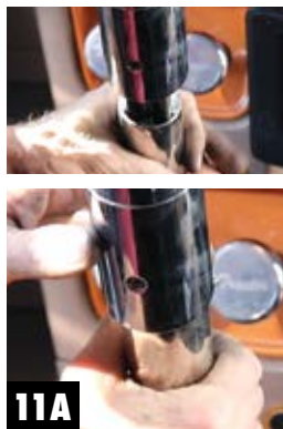
Step 11 Slide Up Shifter Sleeve • Slide up the shifter sleeve to the base cover (See Fig. 11A). Tighten the screw with a 3/32 inch Allen wrench (11B).
