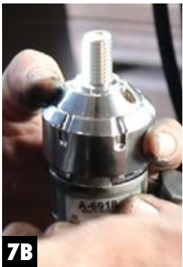
Step 7 Connect Speed Shift Adapter • Connect the RWC adapter to the splitter and install provided screws with 3/64" Allen Wrench (See Fig. 7A & 7B). NOTE: Test levers to make sure they move properly.
