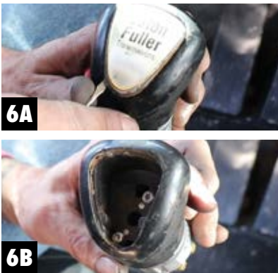
Step 6 Remove Shifter Knob • Using a flat head screwdriver, pop off the cap of the handle (See Fig. 6A). Then use a Torx T20 bit to remove the screws (6B).
