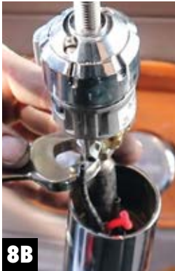
Step 8 Attach Adapter / Splitter • Twist on splitter (8A). Then tighten the jam nut to the splitter with the 3/4" wrench while holding onto the adapter (8B).
