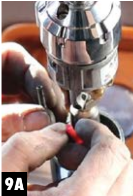
Step 9 Reattach the Air lines to the Splitter. • The air lines are push connects. It is recommended to use two needle nose pliers. Put one on the line and one on the fitting collar. Then push together (See Fig. 9B & 9C). NOTE: Pull down hard on the air lines to make sure they are secure.
