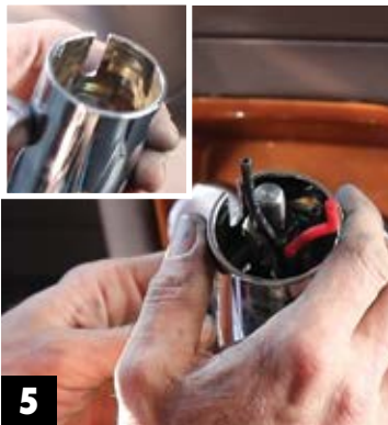
Step 5 Install Base Cover • Slide on the RWC Gearshift Base Cover. NOTE: Make sure that the cut-out is at the top for the shifter lever.
