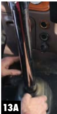
Step 13 Fix Shifter Skirt • Pull up the shifter skirt to cover the bottom of the stainless sleeve (See Fig. 13A & 13B).
