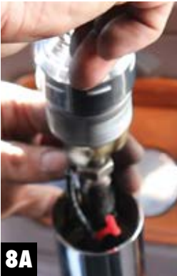
Step 8 Attach Adapter / Splitter • Twist on splitter (8A). Then tighten the jam nut to the splitter with the 3/4" wrench while holding onto the adapter (8B).
