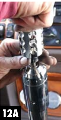
Step 12 Add Shifter Handle • Thread on a RWC Billet Shifter Handle (See Fig. 12A & 12B).
