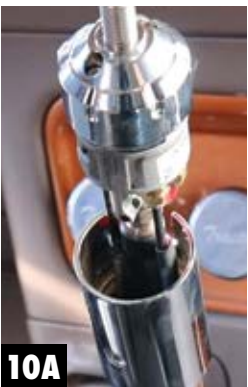
Step 10 Slide Up the Base Cover • Slide up the base shift cover (See Fig. 10A & 10B). Install the 2 Torx T20 screws that were taken out of the old base cover (10C).
