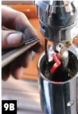
Step 9 Reattach the Air lines to the Splitter. • The air lines are push connects. It is recommended to use two needle nose pliers. Put one on the line and one on the fitting collar. Then push together (See Fig. 9B & 9C). NOTE: Pull down hard on the air lines to make sure they are secure.
