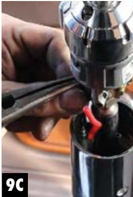
Step 9 Reattach the Air lines to the Splitter. • The air lines are push connects. It is recommended to use two needle nose pliers. Put one on the line and one on the fitting collar. Then push together (See Fig. 9B & 9C). NOTE: Pull down hard on the air lines to make sure they are secure.
