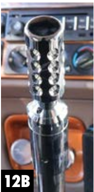
Step 12 Add Shifter Handle • Thread on a RWC Billet Shifter Handle (See Fig. 12A & 12B).
