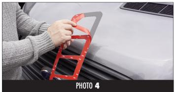
**STEP 4—Removing Backing From Double-sided Tape** Carefully remove the backing from the double-sided tape from one of the overlays. (See Photo 4)
