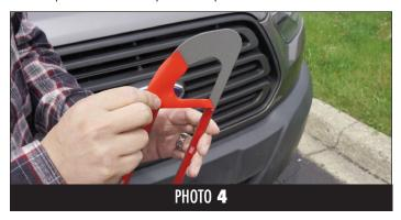
**STEP 4 — Removing Backing From Double-sided Tape** Beginning with the top grille overlay, carefully remove the backing from the doublesided tape. (See Photo 4)
