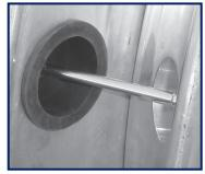
3. If possible, check between the duals to make sure the flange of the stabilizer has come through the hole in the back side of the wheel and is seated around it.
