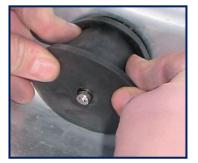
Continue pushing the rubber stabilizer into the wheel hole until the stabilizer's front face is completely seated onto the face of the wheel.
