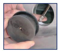
Place the rubber valve stem stabilizer up to the valve extension, and align the stabilizer's center hole with the valve extension tip.
