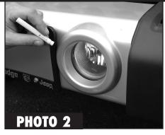
2. Important: Prime only the plastic area where the Fog Light Surrounds are to be installed. After the areas are completely cleaned and dry, you must then coat these plastic areas with 3M Tape Primer 94 (included). Thoroughly coat the cleaned area where the trim is to be installed with the Primer 94 and wait 5 minutes before installing the Trim Piece.
