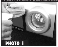
1. Extremely Important: Clean the area where the Fog Light Surrounds are to be installed. If the area where the trim accessory is to be installed is not clean, dry, and free of any vinyl dressing, the trim accessory piece will not stick in place. Begin by cleaning the area thoroughly with a good non-residue cleaner such as Windex, or just clean thoroughly with soap and water and dry completely. Note: Do not use the 3M Tape Primer as a cleaner.
