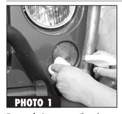
**Extremely Important:** Clean the area where the trim is to be installed. If the area where the trim accessory is to be installed is not clean, dry, and free of any vinyl dressing, the trim accessory piece will not stick in place. Begin by cleaning the area thoroughly with a good non-residue cleaner such as Windex, or just clean thoroughly with soap and water and dry completely. **Note:** Do **not** use the 3M Tape Primer as a cleaner.
