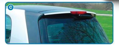
Add a touch of class! A thin band of quality 304 laser-cut stainless steel is used to enhance the rear view of your new Smart, along the top roofline. When the light reflects from this part, they'll have to take a second look.
