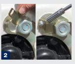
Insert bracket locking tabs into the cavity of the bracket base. Thread nut onto the threaded bolt.
