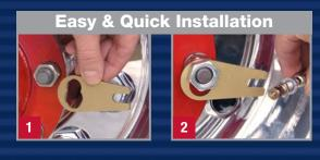
**EZ-Access Air Valve Extension** Kit makes it easy to check tire pressure. Braided stainless steel extensions mount securely to the EZ-Access Air Valve Tabs.
